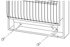
Figure 12 - Installing Bottom Mounting Screws
